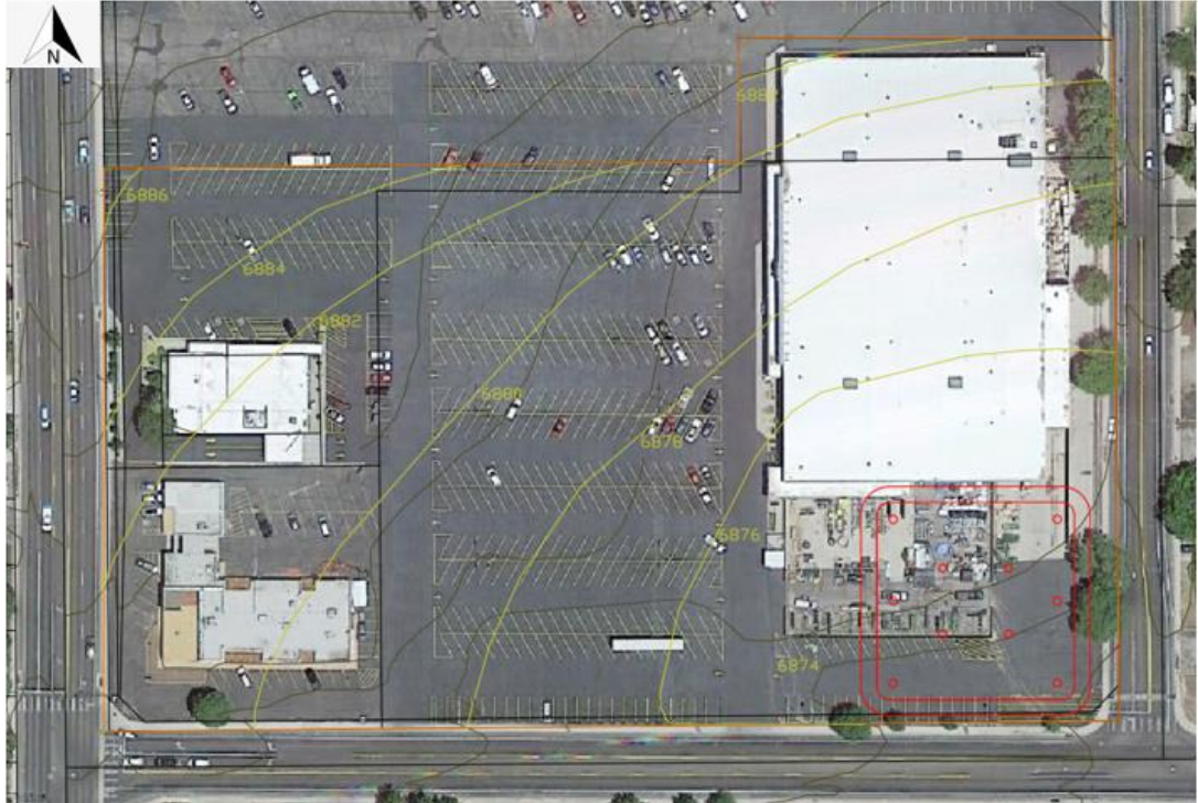
Figure 9: Plan of Retention Basin, Developed Topography, and Drywells in Relation to Existing Parcel
